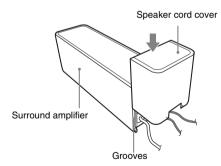
Push the speaker cord cover down until you hear a click. Turn the surround amplifier upside down, then store the cords in the speaker cord cover. 2 Insert the tabs of the speaker cord holder in the slots of the speaker cord cover, and press it into place.
